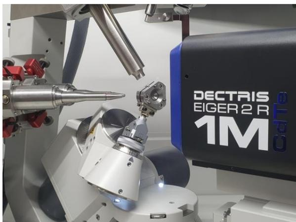
**Figure 1.** A Merrill-Bassett diamond anvil cell during a single-crystal X-ray diffraction measurement employing Ag K $\alpha$  radiation.
